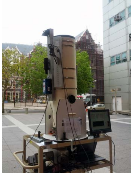
Mid-IR Lidar at 4.5 microns
