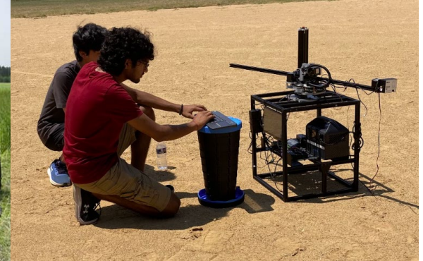
RHG-BRDF measurement system
