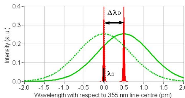
**Figure 3-5:** Wavelength spectra for the backscattered Mie (red) and Rayleigh (green) signal for a 355 nm source at  $\lambda_0$  (dotted lines) and a Doppler shift  $\Delta\lambda_0$  (bold lines); the indicated Doppler shift of 0.5 pm corresponds to a LOS wind speed of  $\sim 200$  ms<sup>-1</sup>.
