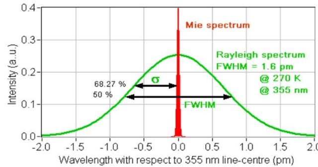
**Figure 3-4:** Wavelength spectra for the backscatter signals from aerosols (Mie spectrum, red) and from molecules (Rayleigh spectrum, green) illustrating the different spectral widths ( $\sigma$ , Full Width Half Maximum FWHM= $2\sqrt{2\ln 2}\sigma$ ) at a laser wavelength of 355 nm for 0 ms<sup>-1</sup> wind speed.
