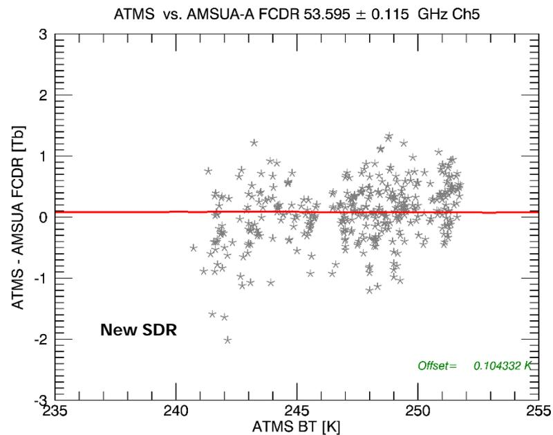
Comparisons show inter-comparison with FCDR is capable of revealing changes in SDR processing. In this case shows change in bias from old version SDR to new version SDR
