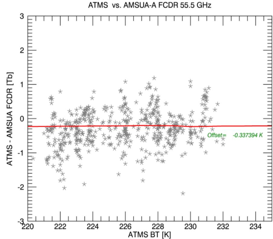
Shows the temperature dependence of bias of ATMS. Close to pre-launch levels (Weng et al, 2016)
