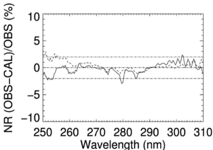
**Figure:** The albedo error versus wavelengths was evaluated via a comparison of measured normalized radiances (referred as NRs OBS) to model calculated normalized radiance (NRs CAL) for specific measurement geometries, viewing conditions and climatological data. The NRs were calculated for a set of given solar zenith and azimuth angles, ozone concentrations, surface pressures, and reflectivity values as inputs to a standard forward radiative transfer model TOMRAD. Results presented in
