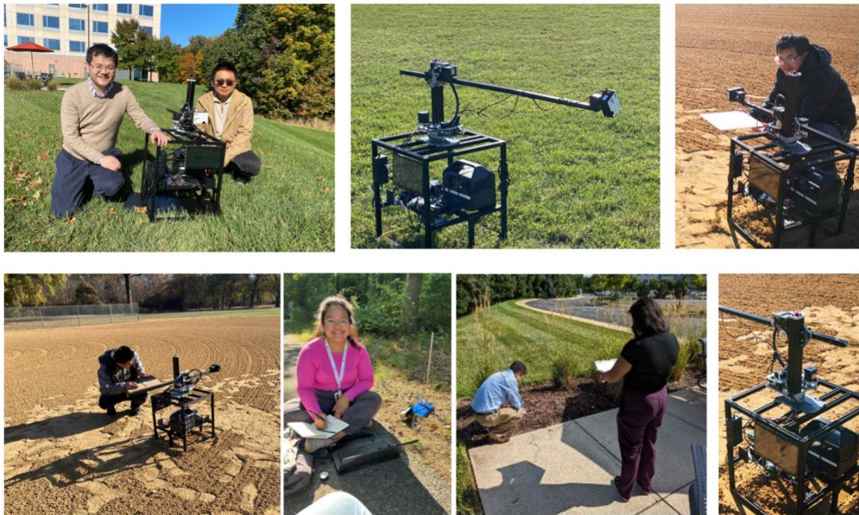
Figure: Field experiments with the RHG-BRDF system over grass, soil and sand scenes and its calibration with a reflectance reference board.
