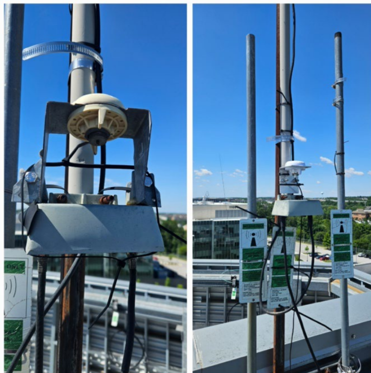
Figure: Damaged GPS antenna (left) and new replacement GPS antenna (right) at the Applied Physics Laboratory, Johns Hopkins University. Image credit: Joseph Patton (CISESS/ESSIC/UMD)
