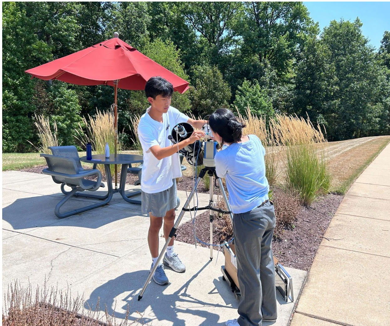
Figure. David Liu and Rosalyn Fang connect an optical fiber cable to an Ocean Insight Spectrometer while setting up a robotic hyperspectral sensor for measurements of the polarization property of atmospheric scattering, 15 July 2024. Image credit: Xi Shao (CISESS)
