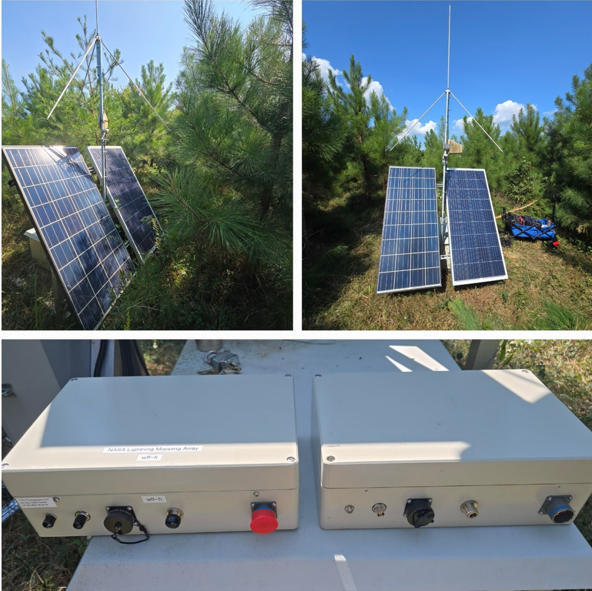
Figure: (Top left and right) The Mid-Atlantic Lightning Mapping Array site at the UMD UAS Test Site before and after tree trimming to unblock the solar panels. (Bottom) The upgraded LMA electronics are shown on the left. Photo credit: Guangyang Fang
