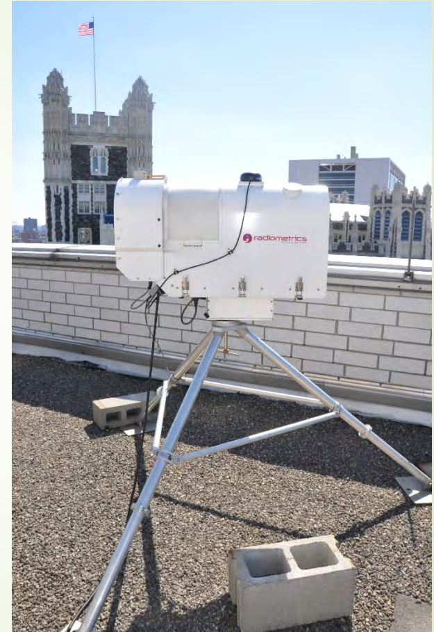
Microwave Radiometer Profile located at Steinman Hall @ CCNY
